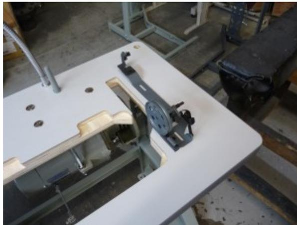
Your thread stand may differ from the one pictured. Assemble the stand by using the coupling to join the two thread stand posts, add the thread stand arms, and attach the thread stand cone platforms to the arms.
