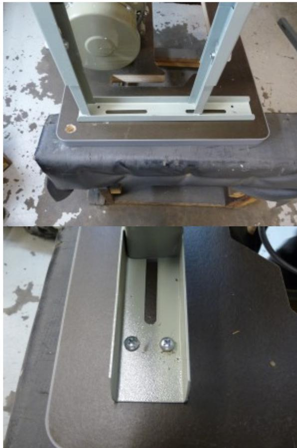
Attach the treadle (motor pedal) to the bottom cross brace as shown in the picture below, centered over the motor.
