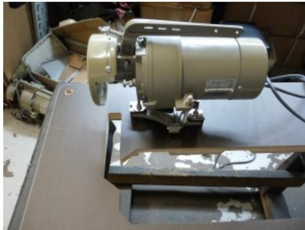
Using the long bolts that came with your motor, tighten down the motor mount to the table.
