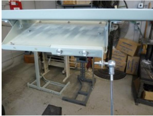
Attach the treadle rod from the treadle to the motors arm.
