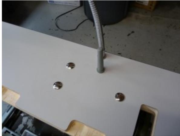
The bobbin winder is installed next to motor belt opening, it may be simpler to install the bobbin winder after the machine has been installed for proper bobbin winder placement.
